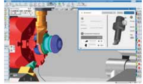
Fig1: The integration of the CoroPlus® Tool Library allows users to define tool assemblies and relevant cutting conditions and import the data directly into GibbsCAM.
