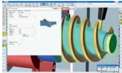
Fig7: Optimised 5-axis stepover for finishing walls and cylindrical or conical floors that creates a better, more consistent surface finish.
