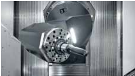
The completely redesigned swivel heads with integrated motor spindles, specially developed by HELLER, contribute significantly to the high accuracy and dynamics of the F 6000.
