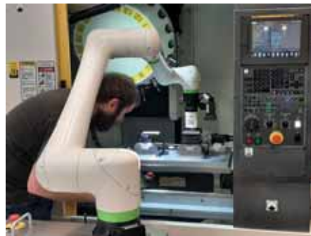
ZiMo flexible robot cell with FANUC cobot serving FANUC ROBODRILL machining centre
