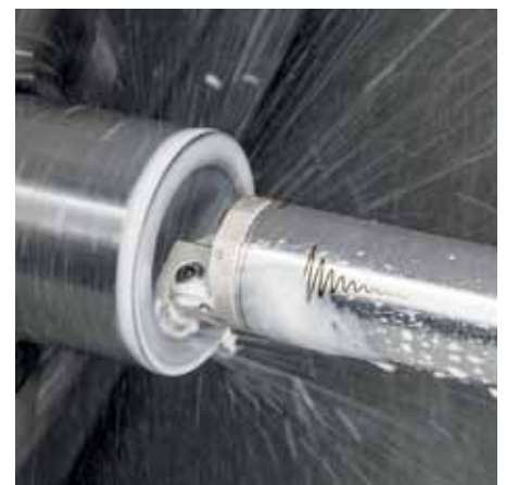
In boring, using anti-vibration bars improves performance and reduces power consumption.
